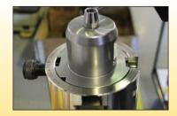
3 Screw the Duo-Lock™ cutting tip into adaptor by hand.
