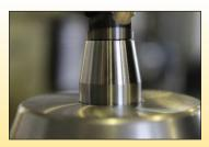
5 Apply the torque shown in the table. Use of a high quality common torque wrench is mandatory. The ERICKSON™ Torque Master wrench is recommended.
