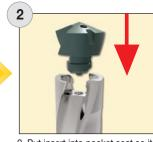
2. Put insert into pocket seat so it rests firmly on the holder.
